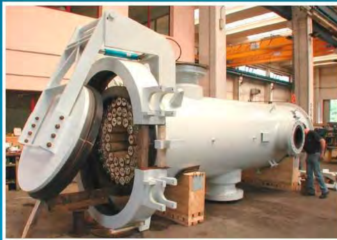
FILTER SEPARATOR SCF TYPE - 63" # 600, THK 56 mm, 30 ton
