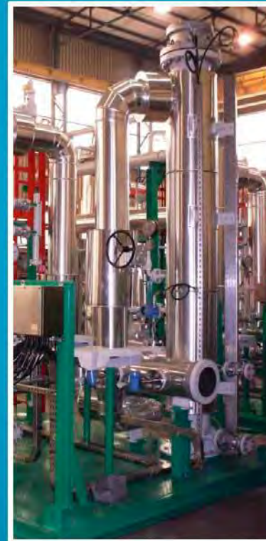
ELECTRIC HEATER RE TYPE 220 KW # 300
