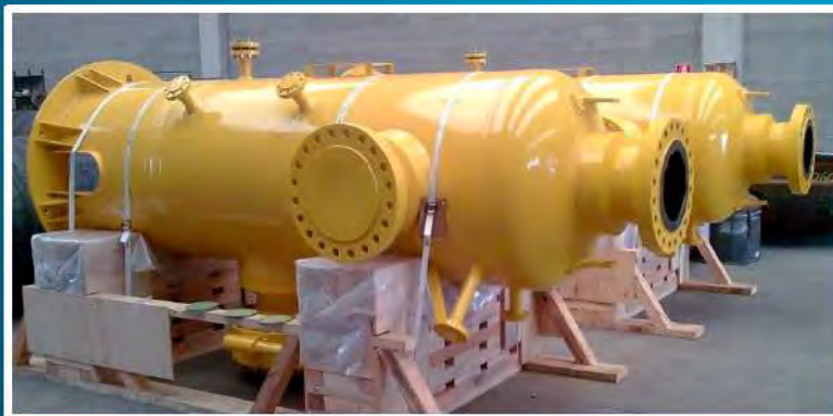
2 SC TYPE MULTITUBE SEPARATORS - 39" # 600
