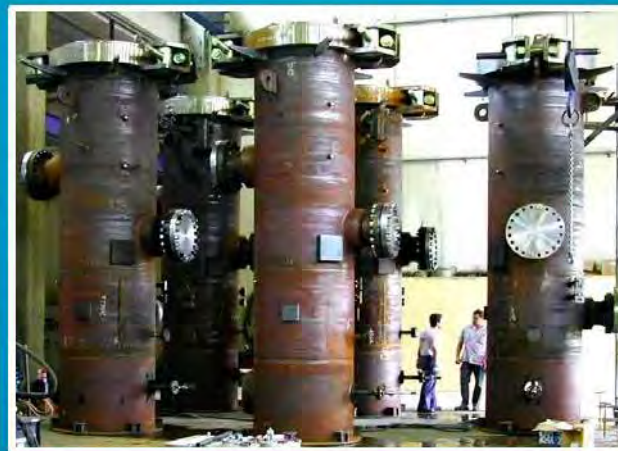
5 FILTER SEPARATORS SCF TYPE - 48" # 600
