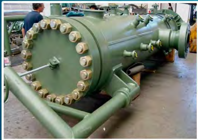
ABSOLUTE SEPARATOR SA TYPE - 44" # 1500 RJ, THK 70 mm, 16 Ton
