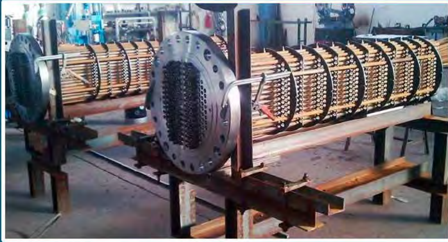
2 HEAT EXCHANGERS BEU TYPE – DUTY 1.500 KW # 600 each
