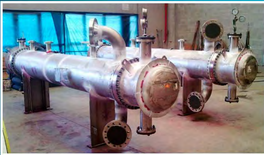
2 HEAT EXCHANGERS BFM TYPE – DUTY 787 KCAL/h # 600 each
